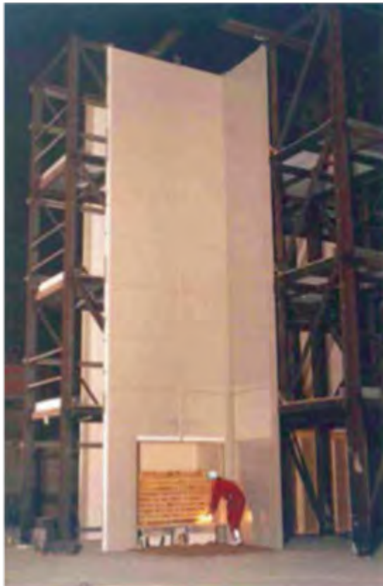
Fig. 7.3 BS8414-2 test rig (from BRE report BR135 [17])
